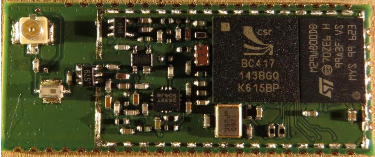
Figure 4: WT41u-E, internal, top view
