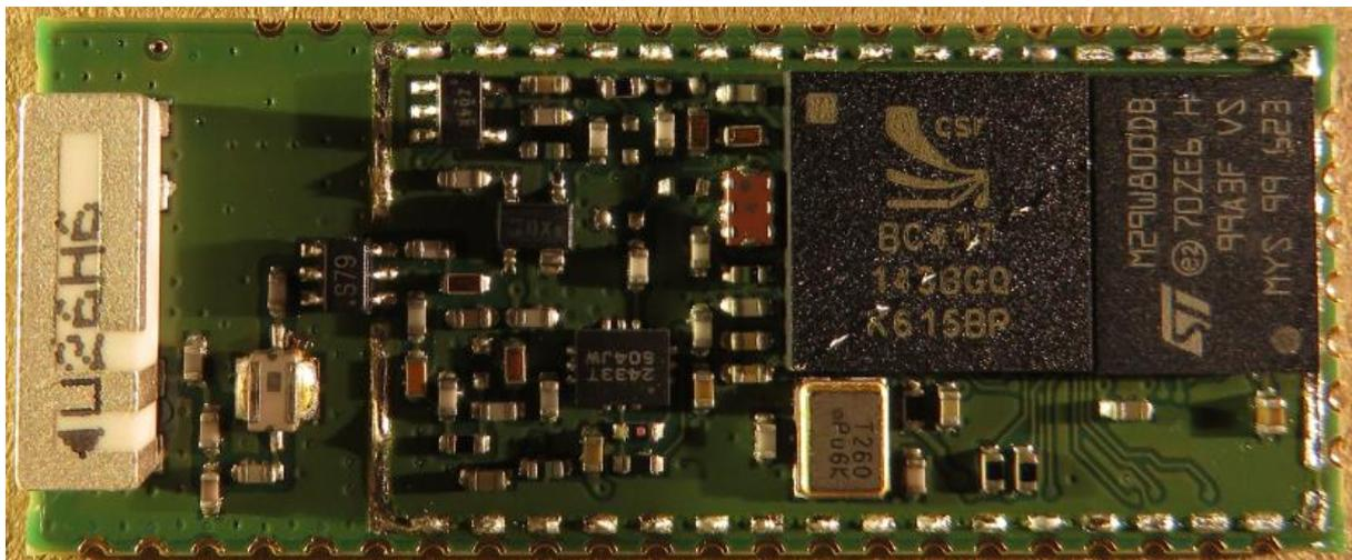
Figure 3: WT41u-A, internal, top view
