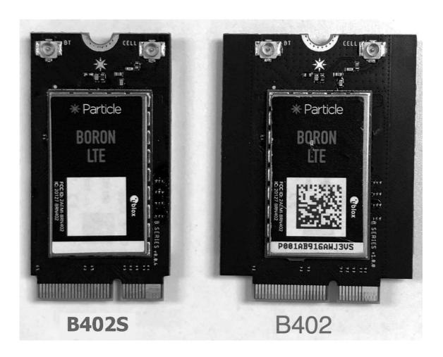
The difference between B402 and B402S is only the width of the edge of the board. The B402S is 22mm wide and the B402 is 30mm wide.
