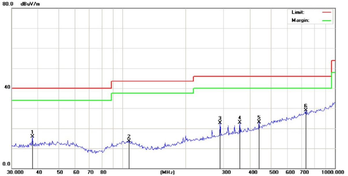
Site: FCC Part 15B Class B RE\_3 m      Polarization: **Horizontal**      Temperature: 23
