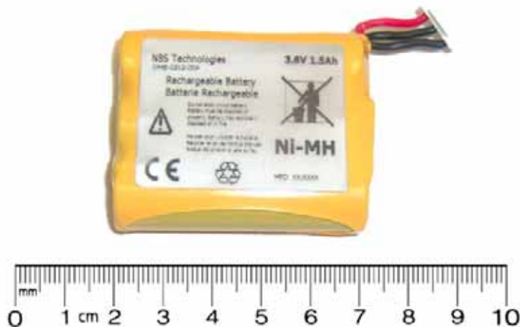
< Rechargeable Ni-MH battery (3.6V, 1.5 Ah) >
