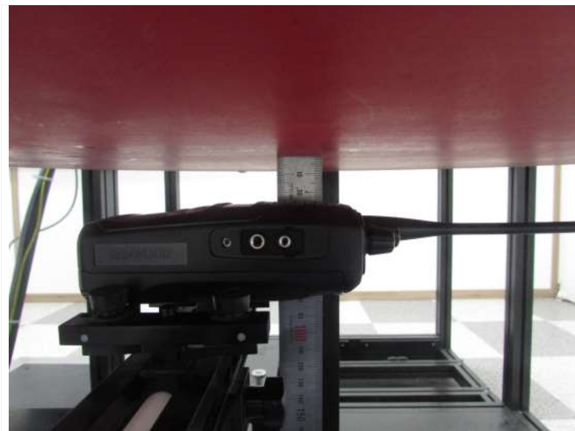
Distance of 25 mm from the EUT
