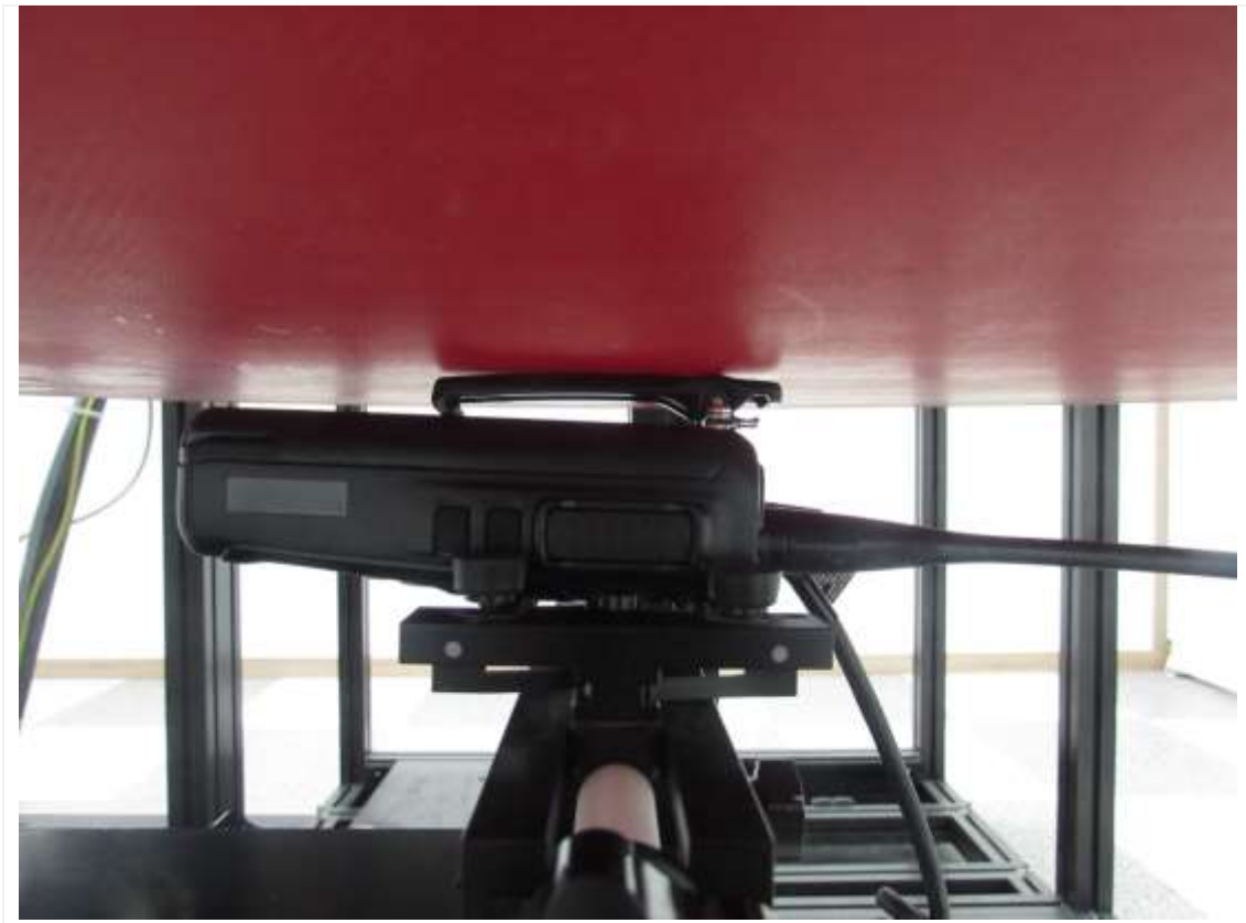
Distance of 0 mm from the EUT
