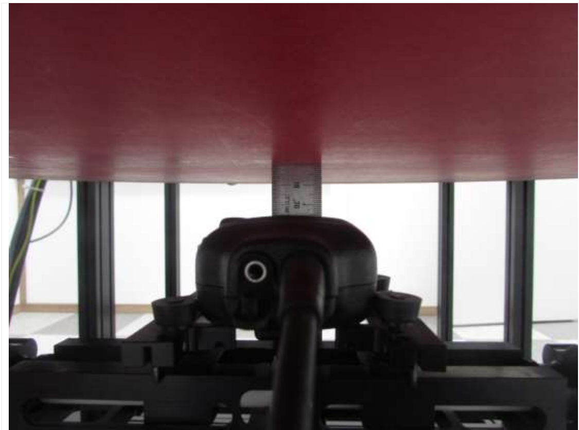
Distance of 25 mm from the EUT
