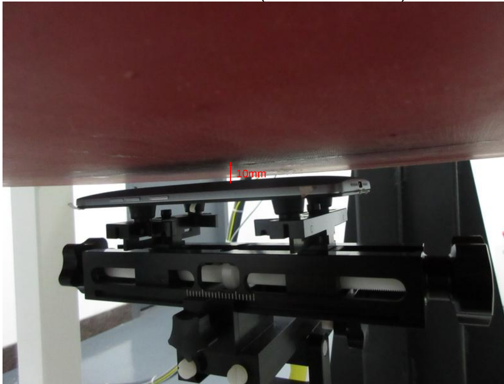
Test Position Rear Face(Test distance=10mm)
