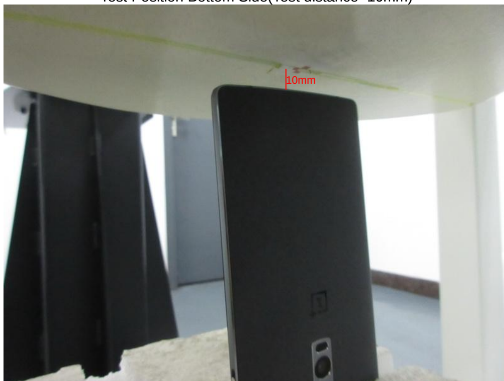
Test Position Bottom Side(Test distance=10mm)
