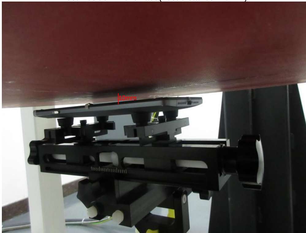
Test Position Front Face(Test distance=10mm)
