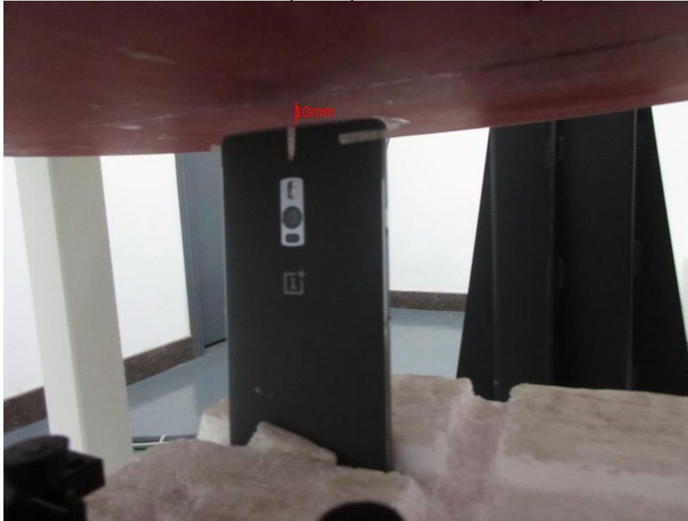
Test Position Top Side(Test distance=10mm)
