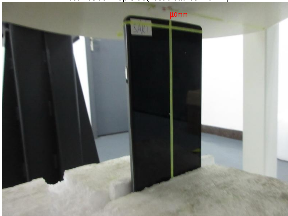
Test Position Top Side(Test distance=10mm)
