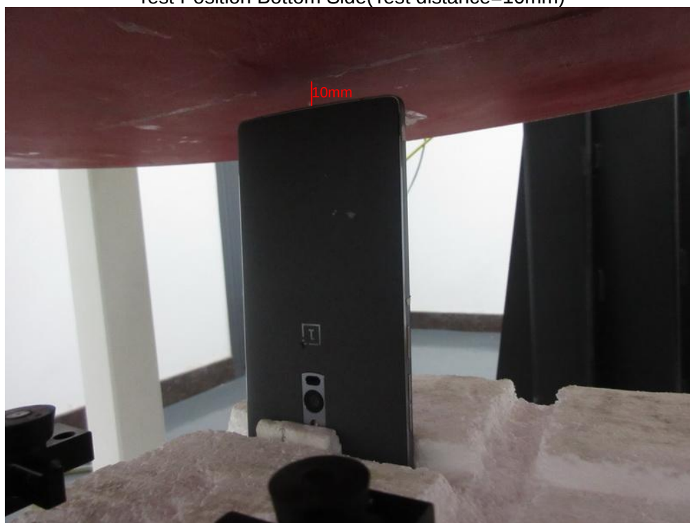
Test Position Bottom Side(Test distance=10mm)
