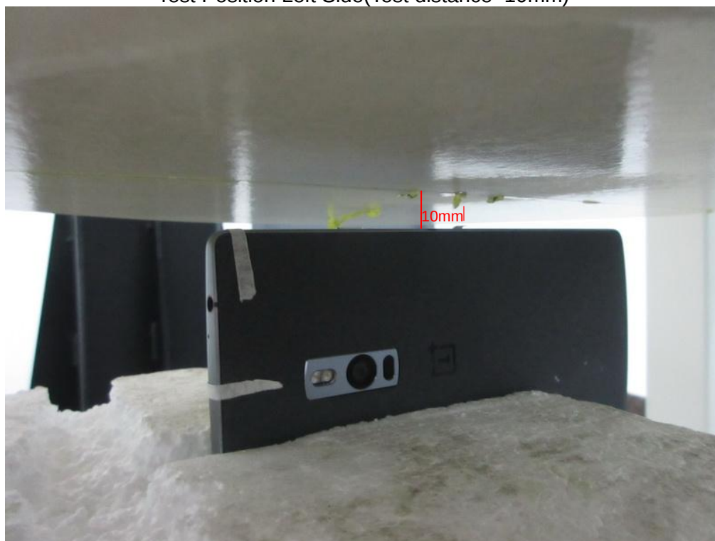
Test Position Left Side(Test distance=10mm)
