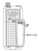
Install Lanvard Install lanyard through attachment points on belt clip.
