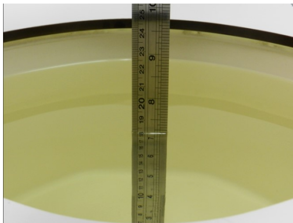
Fig 11.2 Photo of Liquid Height for Body SAR
