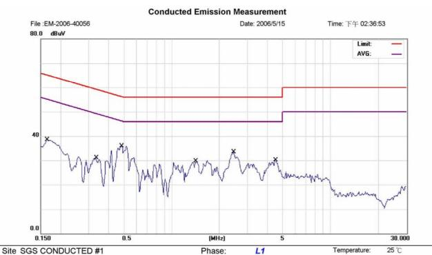
Limit: CISPR22 Class B Conduction(QP)
