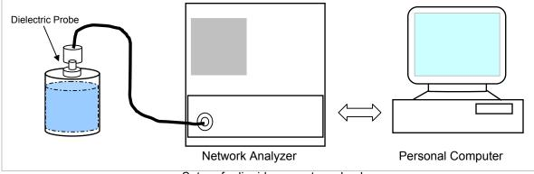
Set-up for liquid parameters check
