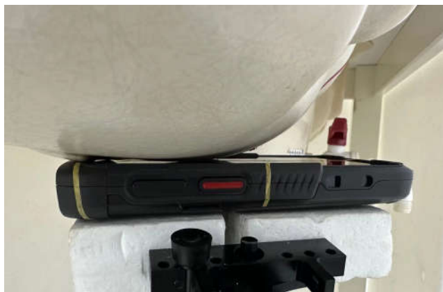
Right Cheek, Test Separation 0 mm
