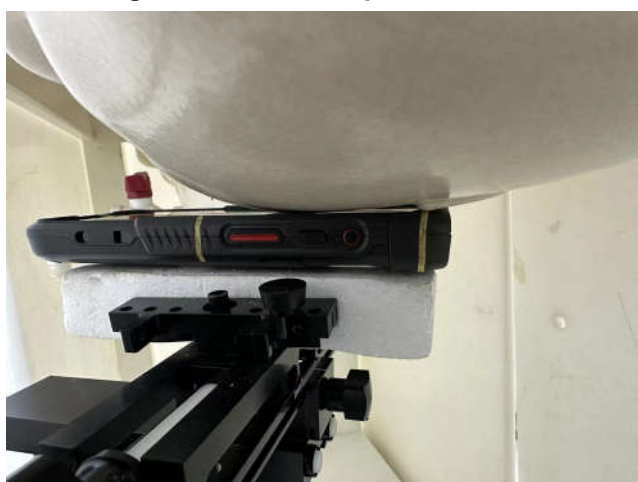
Left Cheek, Test Separation 0 mm
