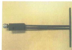
Figure 1 – MVG COMOSAR Validation Dipole
