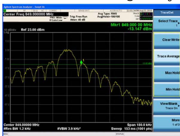
NB-IOT Band 26 QPSK 3.75kHz 1@47 CH-High
