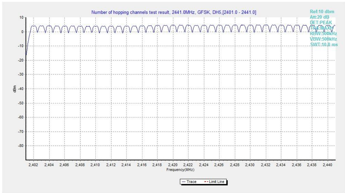
Fig.93. Number of hopping frequencies: GFSK, Channel 0 - 39
