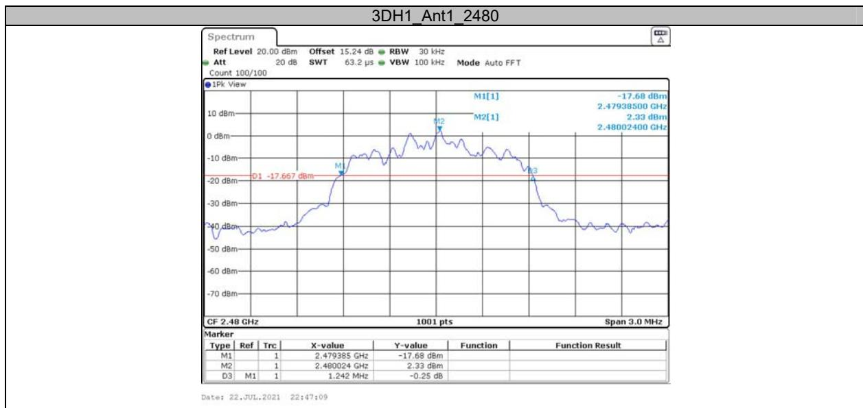
**Appendix B: Occupied Channel Bandwidth****Test Result**
