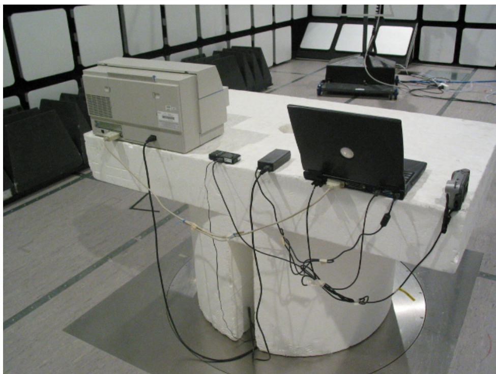
Picture 3 Radiated emission measurement (GSM 1900+Data peripherals)
