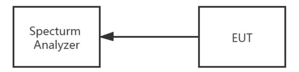
The EUT which is powered by the DC 5V, is connected to the Spectrum Analyzer; the RF load attached to the EUT antenna terminal is 50 Ohm; the path loss as the factor is calibrated to correct the reading. Make the measurement with the spectrum analyzer's resolution bandwidth(RBW) = 100 kHz. In order to make an accurate measurement, set the span greater than RBW.
