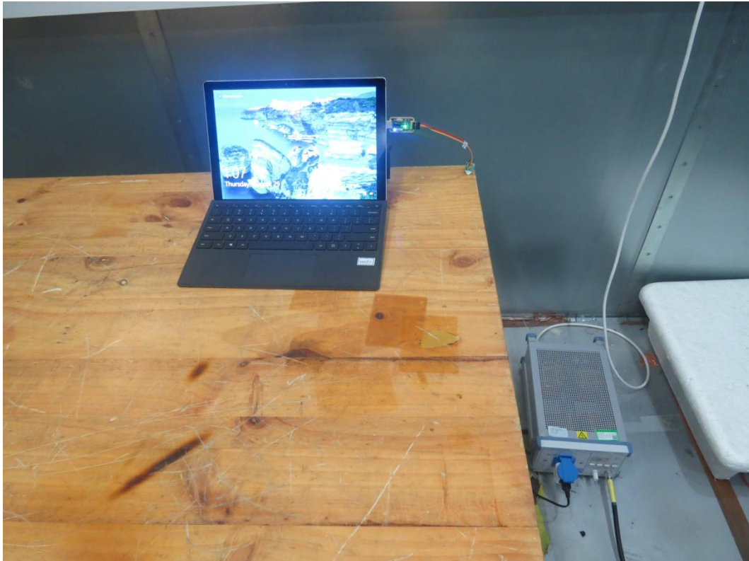
Picture 2 Conducted Emission Test Setup
