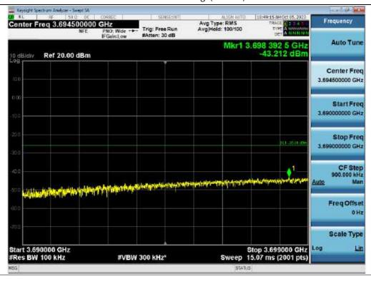
Spurious / 3.7 GHz Service(High) + 3.45 GHz Service(Low) (ANT 1) / Downlink / 5G NR 20 MHz / High Edge(3.7 GHz) ~ High Edge(3.7 GHz) + 10 MHz
