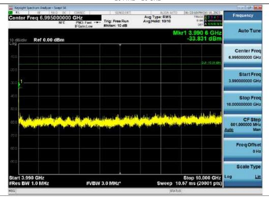
Spurious / 3.7 GHz Service(Low) + 3.45 GHz Service(High) (ANT 2) / Downlink / 5G NR 20 MHz / 10 GHz ~ 40 GHz
