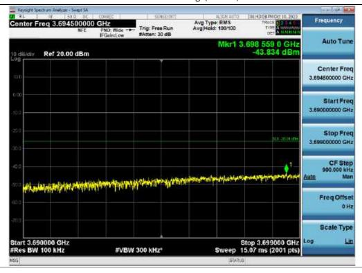
Spurious / 3.7 GHz Service(High) + 3.45 GHz Service(Low) (ANT 2) / Downlink / 5G NR 20 MHz / High Edge(3.7 GHz) ~ High Edge(3.7 GHz) + 10 MHz
