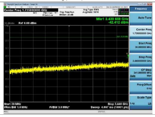
Spurious / 3.7 GHz Service(High) + 3.45 GHz Service(Low) (ANT 2) / Downlink / 5G NR 20 MHz / Low Edge(3.45 GHz) - 10 MHz ~ Low Edge(3.45 GHz)
