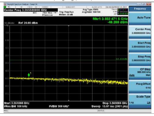
Spurious / 3.7 GHz Service(High) + 3.45 GHz Service(Low) (ANT 2) / Downlink / 5G NR 20 MHz / High Edge(3.45 GHz) + 10 MHz ~ Low Edge(3.7 GHz) - 10 MHz
