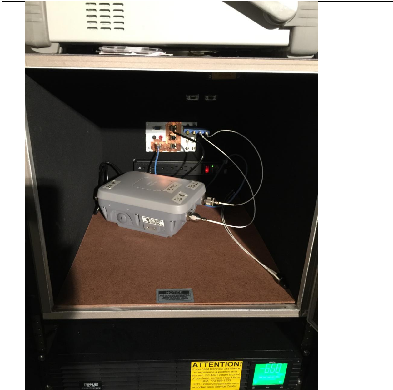
Title: AIR-CAP1532E-B-K9 Conducted Test Setup
