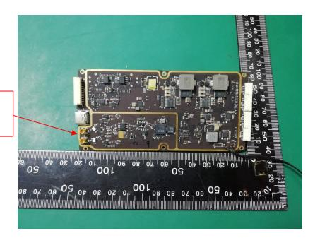
900MHz/2.4GHz image transmission antenna port
