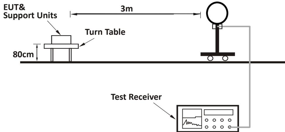
For Radiated emission 30MHz to 1GHz:
