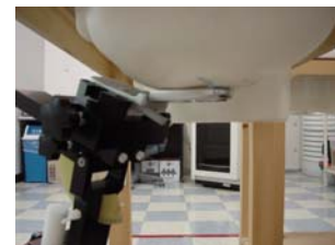
Fig. 16. Head SAR Test Setup
