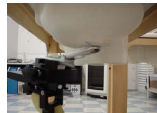
Fig. 18. Head SAR Test Setup
