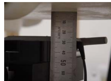
Fig. 22. Body SAR Test Setup with Holster
