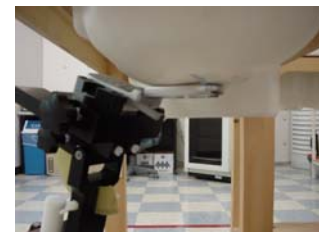
Fig. 15. Head SAR Test Setup
