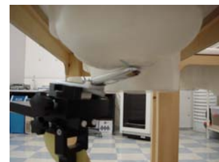
Fig. 19. Head SAR Test Setup
