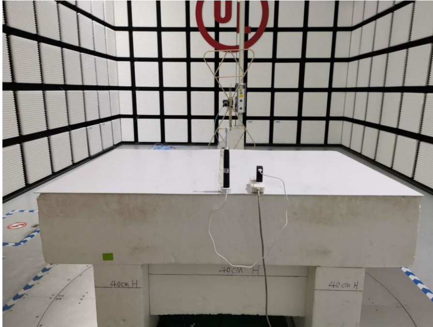
Radiated Emissions below 1 GHz test setup photo
