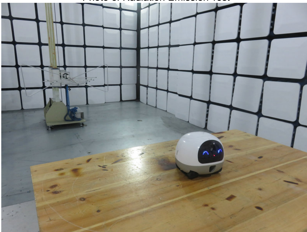
Photo of Radiation Emission Test
