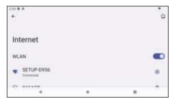
For additional Network detail information's (IP address, Security, Frequency and Advanced), tap setting of the network (e.g. SETUP\_D956).
