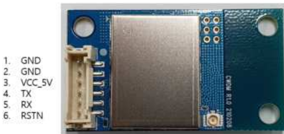
[Fig.3] I/O Interface Connector
