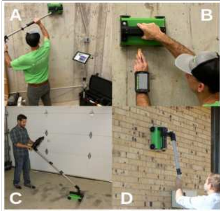
Figure 2: Different smart phone and tablet setups can be used for different survey types: A) Extension handle with tablet on floor stand, B) wrist-mounted smartphone, C) Extension-handle mounted tablet, D) Extension handle.
