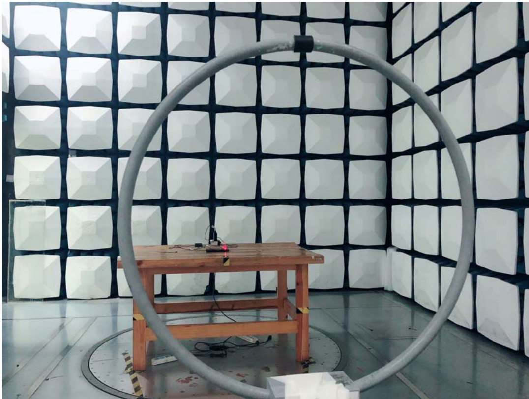
Radiated Emissions –Above 30MHz
