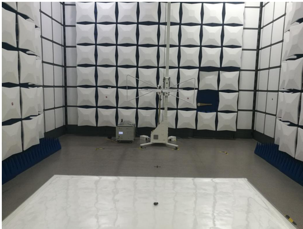
FCC RADIATED EMISSION TEST SETUP
