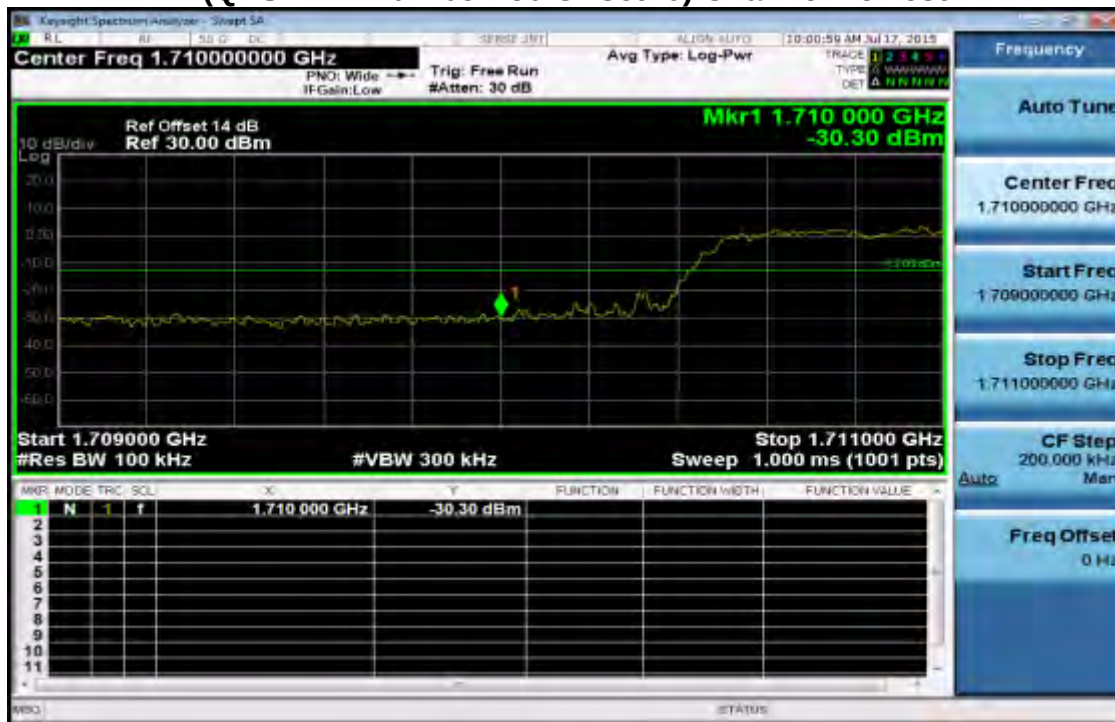
Figure 9-88: Band edge emission at antenna terminals –10MHz BW LTE-Band 4 (QPSK RB Number: 50 Offset: 0) Channel Highest
