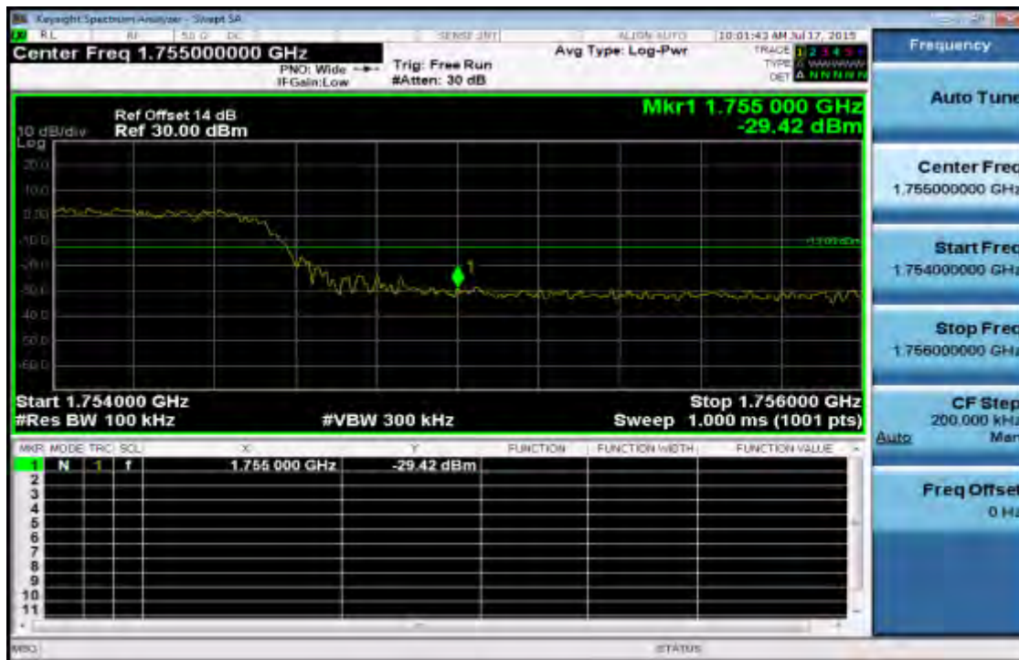
Figure 9-88: Band edge emission at antenna terminals –10MHz BW LTE-Band 4 (QPSK RB Number: 50 Offset: 0) Channel Highest
