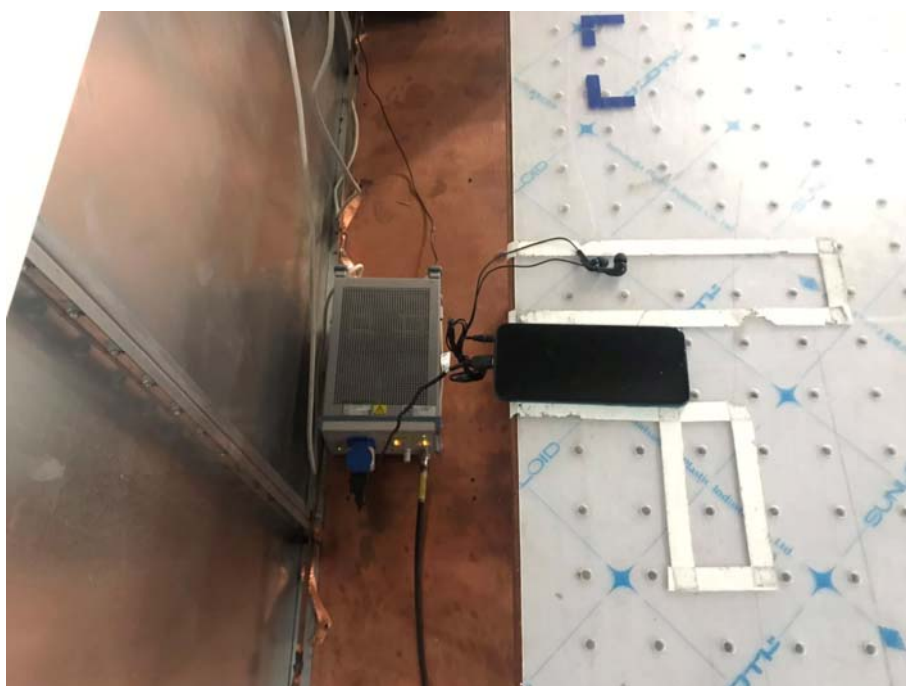
Conducted Emissions Test Setup (with charger)
