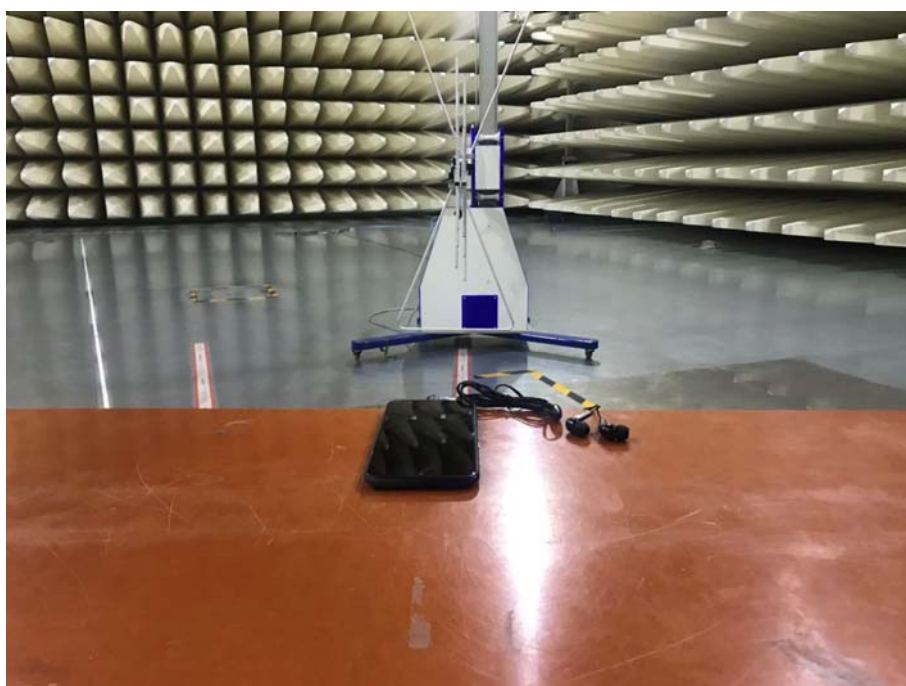
Radiated Emissions Test Setup (with charger) (30-1000MHz)
