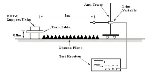
The radiated emission tests were performed in the 10 meters chamber test site for the range 30MHz to 1GHz and the 3 meters chamber test site for above 1GHz, using the setup accordance with the ANSI C63.4-2014. The specification used was the FCC Part 15.109 Class B limits.
