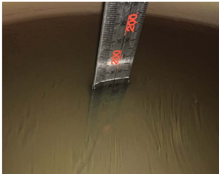
Liquid depth for SAR Measurement
