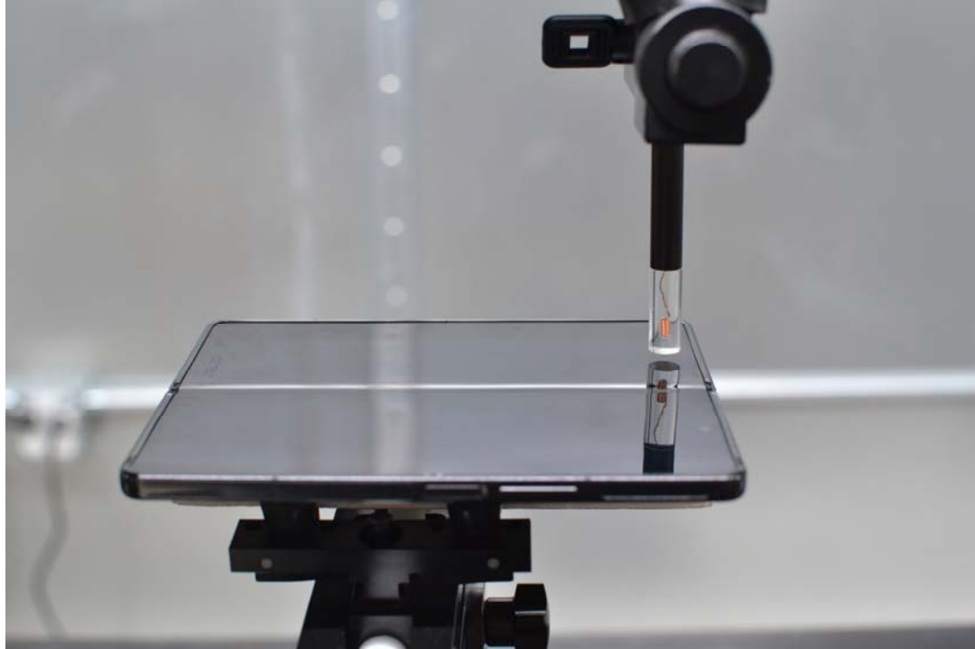
Figure 17-3 Test Setup for Wireless Device - OPEN (FRONT)
