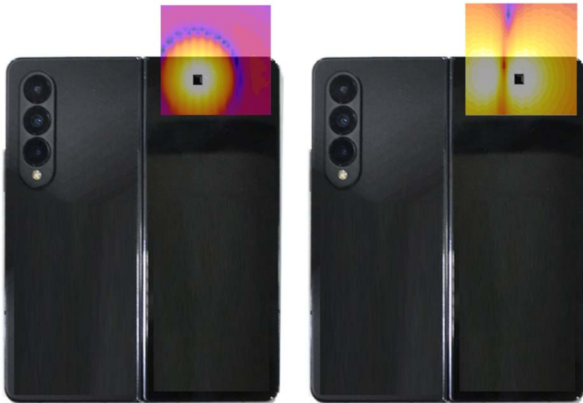
Figure 17-9 T-Coil Scan Overlay Magnetic Field Distributions (OPEN – BACK)
