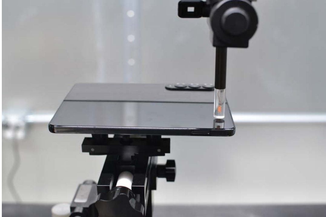
Figure 17-5 Test Setup for Wireless Device - OPEN (BACK)
