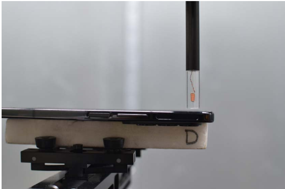
Figure 17-4 Test Setup for Wireless Device - OPEN (FRONT)
