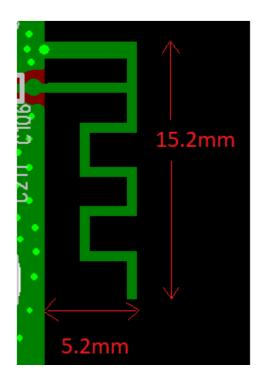
Figure 1 Physical dimension (mm)
