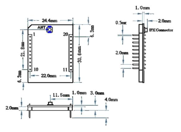
Pin Order: From PIN1 to PIN20, Anticlockwise.
