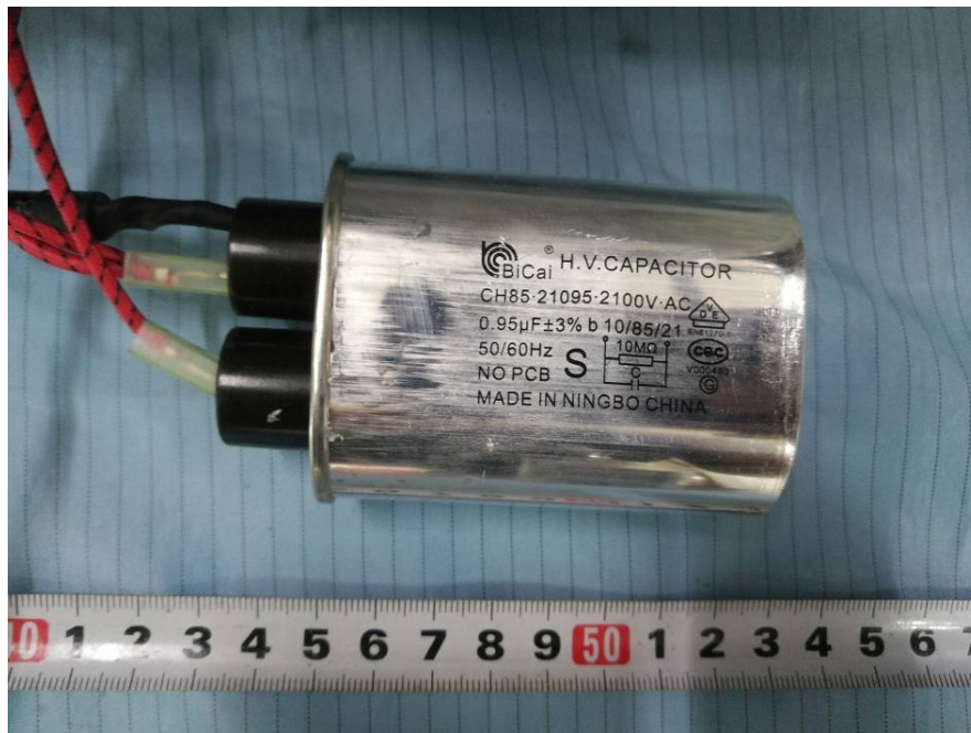
EUT – High Voltage Capacitor View
