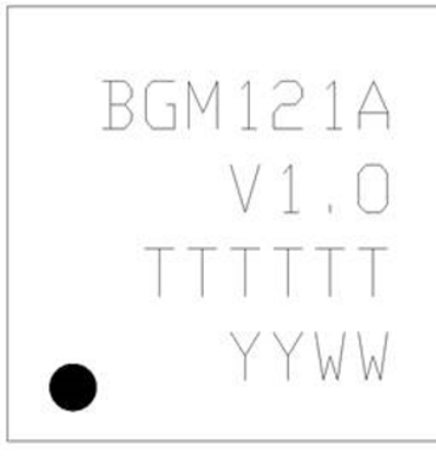
Figure 8.4. BGM121/BGM123 Package Marking
