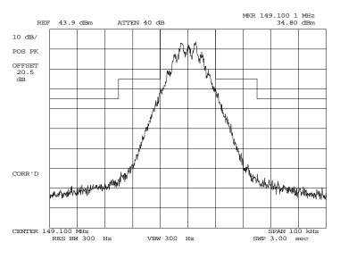
POWER: MODULATION: HIGH GMSK 19200 BITS PER SECOND MASK: B, VHF/UHF 25kHz, w/LPF
