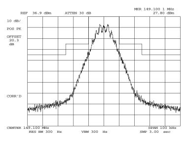
POWER: MODULATION: LOW GMSK 19200 BITS PER SECOND MASK: B, VHF/UHF 25kHz, w/LPF
