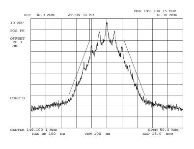
POWER: MODULATION: LOW GMSK 9600 BITS PER SECOND MASK: D, VHF/UHF 12.5kHz BW
