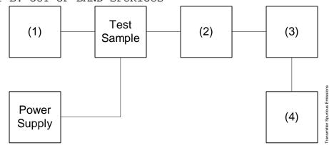
Asset Description s/n (as applicable) (1) <u>AUDIO OSCILLATOR/GENERATOR</u> i00010 HP 204D 1105A04683 i00017 HP 8903A 2216A01753 i00012 HP 3312A 1432A11250 (2) COAXIAL ATTENUATOR i00122 Narda 766-10 7802 i00123 Narda 766-10 7802A i00069 Bird 8329 (30 dB) 1006 i00113 Sierra 661A-3D 1059 (3) FILTERS; NOTCH, HP, LP, BP
