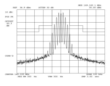
POWER: MODULATION: LOW VOICE: 2500 Hz SINE WAVE MASK: B, VHF/UHF 25kHz, w/LPF
