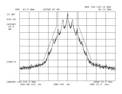
POWER: MODULATION: HIGH GMSK 9600 BITS PER SECOND MASK: D, VHF/UHF 12.5kHz BW
