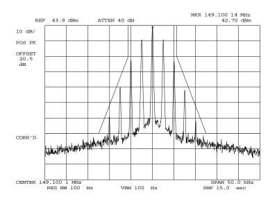
POWER: MODULATION: HIGH VOICE: 2500 Hz SINE WAVE MASK: D, VHF/UHF 12.5kHz BW
