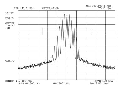
POWER: MODULATION: HIGH VOICE: 2500 Hz SINE WAVE MASK: B, VHF/UHF 25kHz, w/LPF
