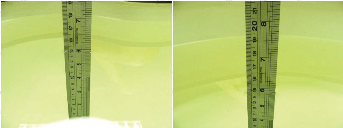
Photo of Liquid Height for Head SAR
