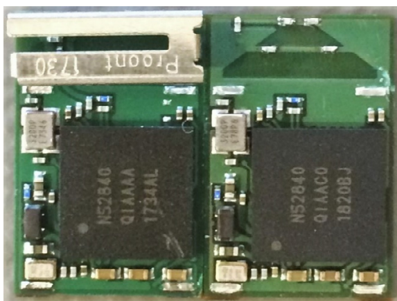
Figure 1: Antenna configuration comparison - NINA-B312 to the left, NINA-B316 to the right
