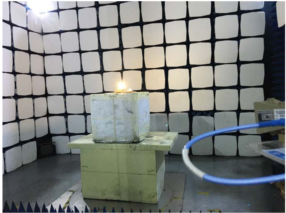
Radiation Emission Test Setup (Above 18GHz)
