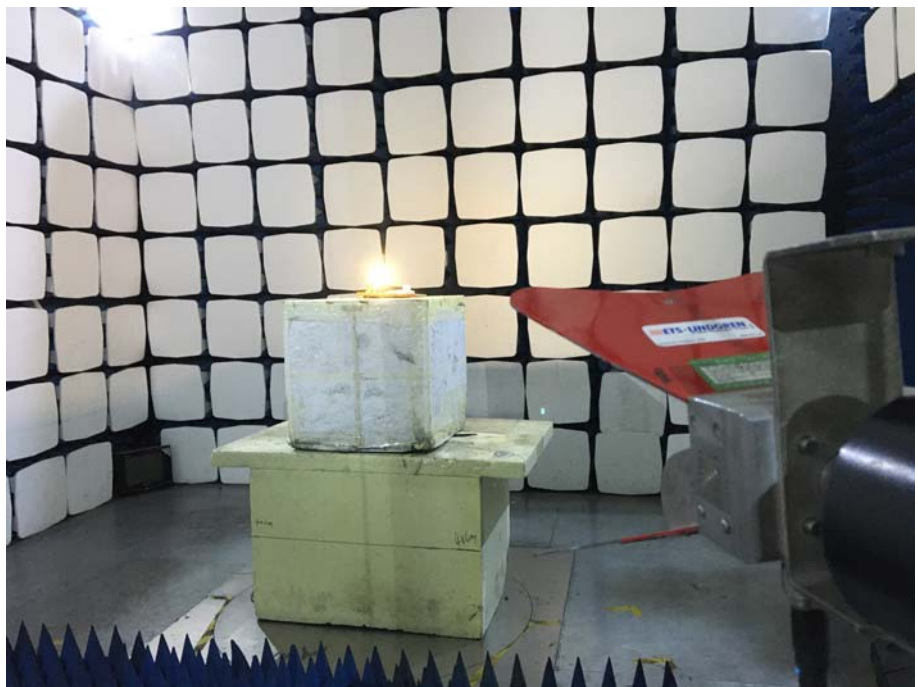
Radiation Emission Test Setup (1GHz to 18GHz)
