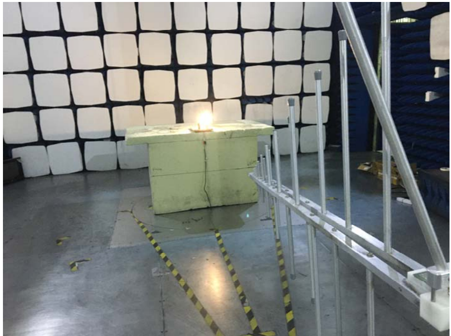
Radiation Emission Test Setup (30MHz to 1GHz)
