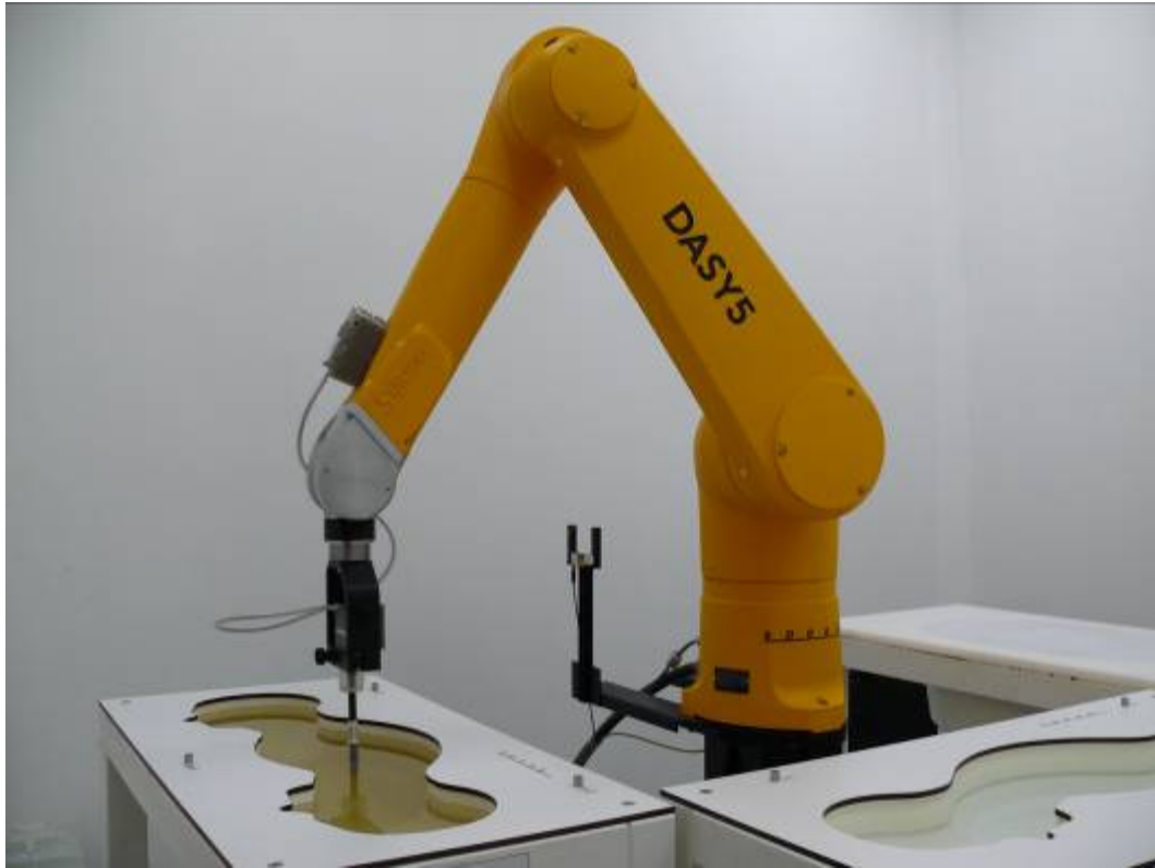
Picture 1: Specific Absorption Rate Test Layout
