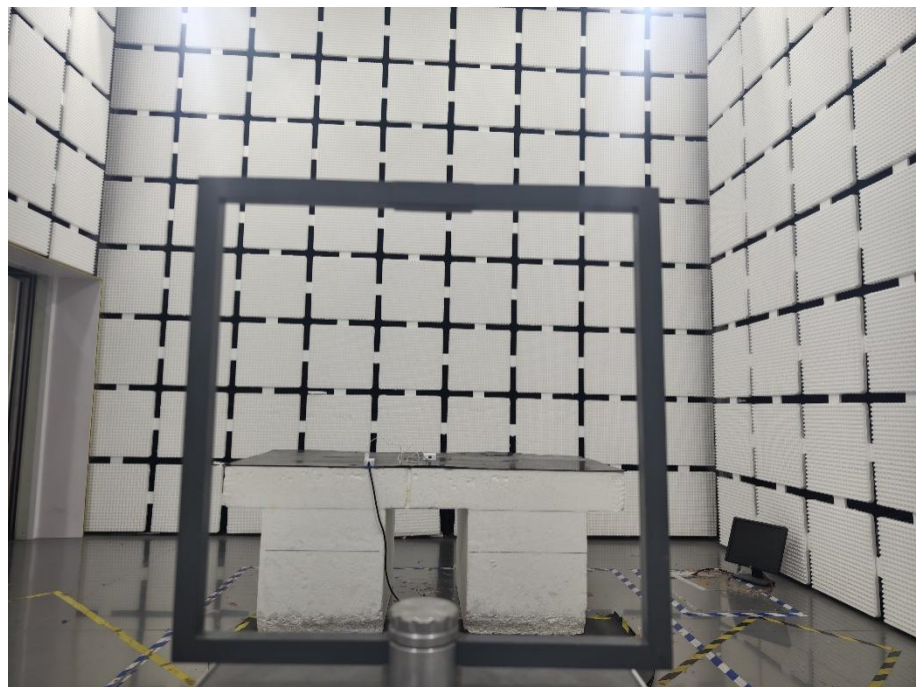
Radiation Emission Test Setup (Below 30MHz)
