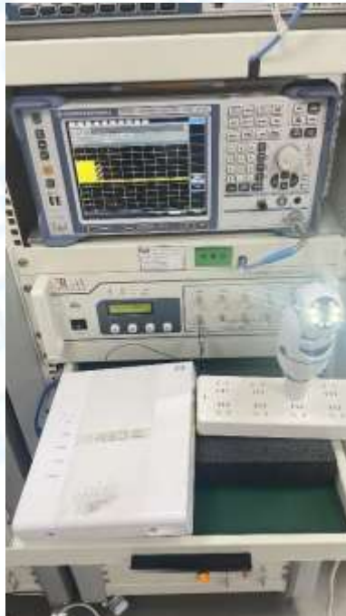
Photo of Setup for DFS Test
