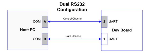
Note that "COM A" and "COM B" labels are used on the host PC in the above diagram. This is to identify the physical COM ports and should not be confused with the COM port number assigned by Windows.
