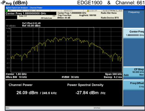
PAPR (dB) = P<sub>Pk</sub> (dBm) - P<sub>Avg</sub> (dBm) = 26.23 dBm - 26.09 dBm = 0.14 dB
