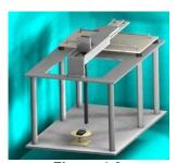
Figure 4-3 RF Near-Field Scanner
