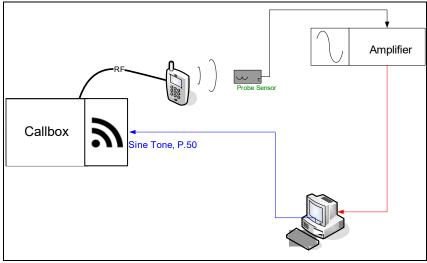
Figure 4-2 **T-Coil Test Setup**
