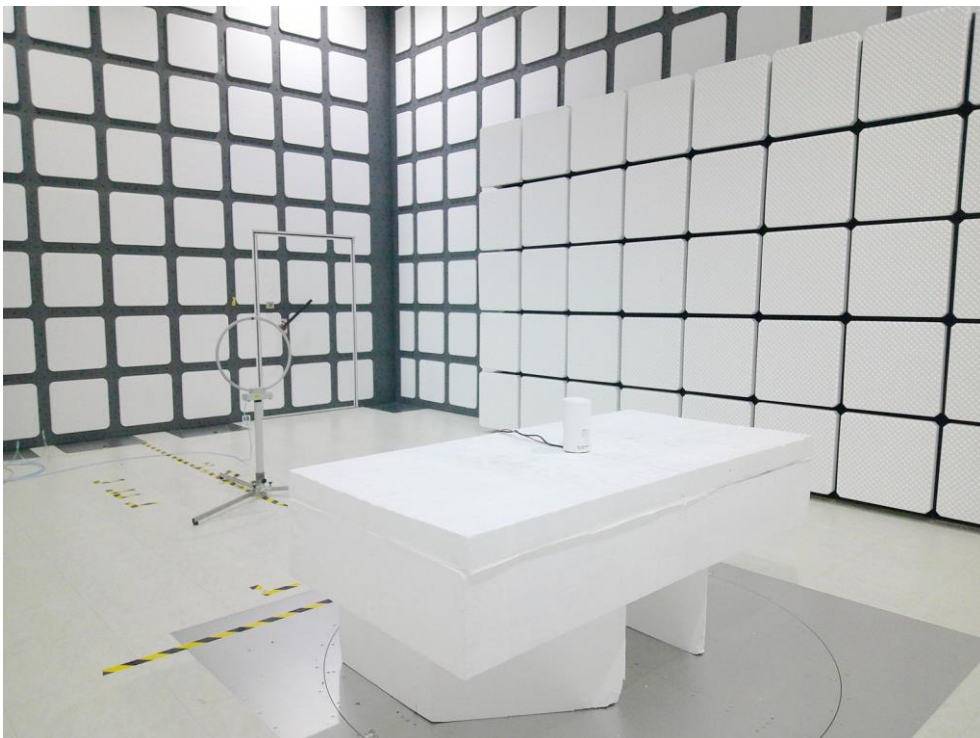
Description: Radiated Emission Test Setup for 9kHz~30MHz
