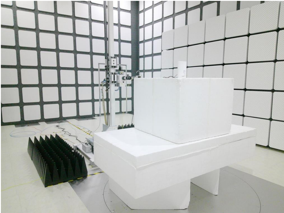
Description: Radiated Emission Test Setup for 9kHz~30MHz
